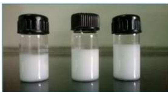
Figure 3: Addition of 2 ml, 3 ml and 5 ml water to the emulsion
