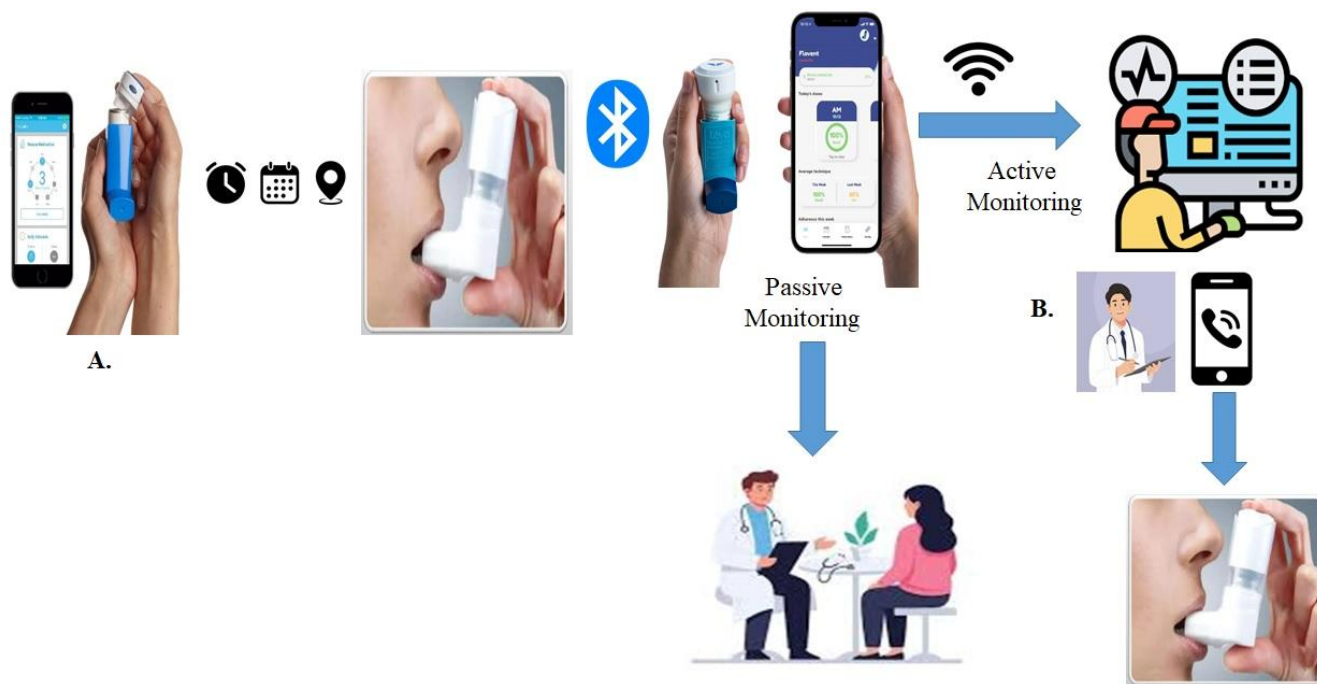
Figure 2: Schematic representation of Digital inhaler platform with connection between patient, inhaler sensors, and healthcare provider. A). Patient self- assessment, record adherence & Inhaler use reminders; B). Personalization of care
